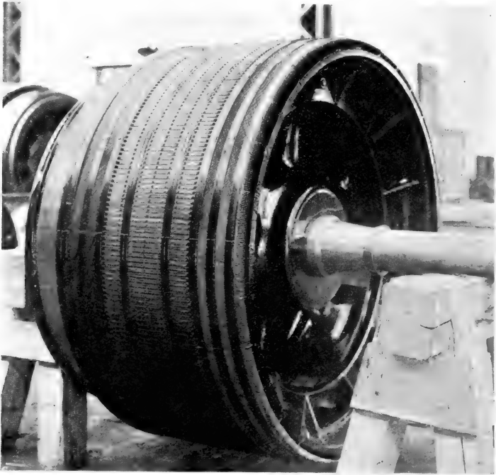
FIG. 320.—Large Armature, showing Equaliser Ring Construction (Union Electric Co. of Berlin).
